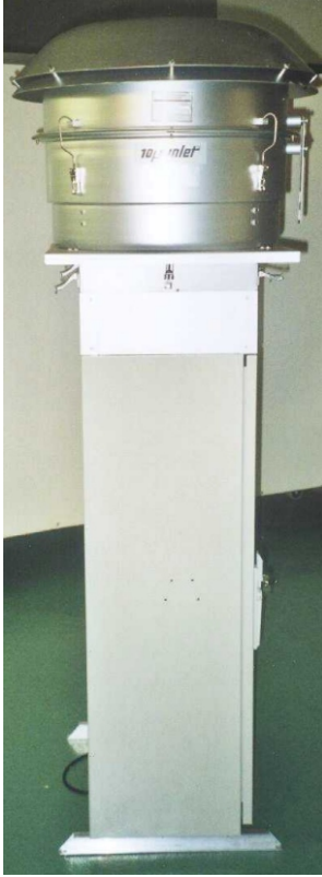
MicroPNS HVS1 with outdoor housing and PM 10 sampling head according EN 12341
