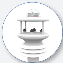
SP276 Weather Station based on GILL module
